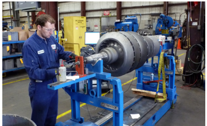
Electrical run-out testing.
