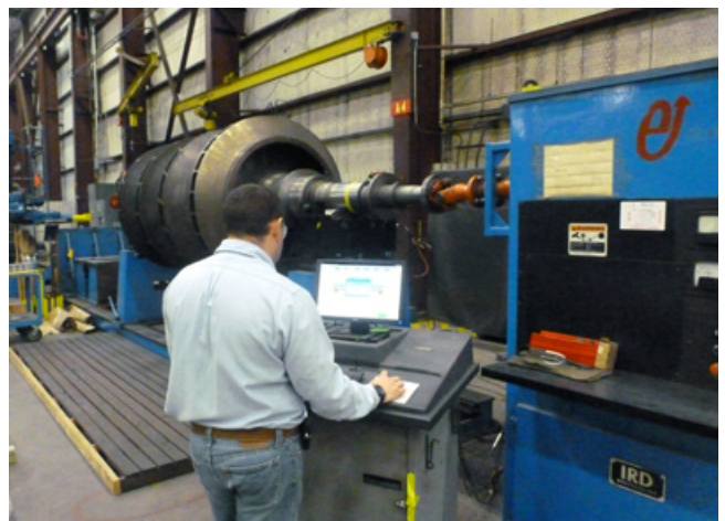
Balancing a large centrifugal compressor rotor.
