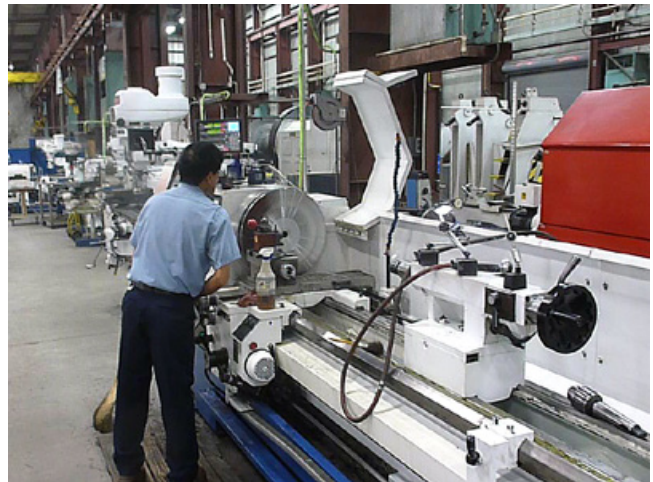
Facing a steam turbine rotor disc in a lathe.
