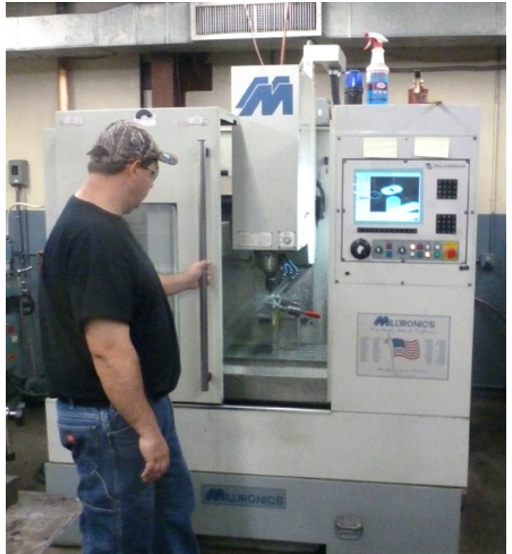
Machining the top of a small bucket in a CNC mill.
