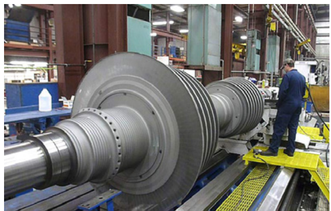
Grinding a 200 MW rotor bearing journal in the 84-inch lathe.
