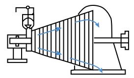
SINGLE-FLOW CONDENSING are highly economical and require the least steam for a given horsepower. Typically, they are directly connected to a high-speed compressor.
