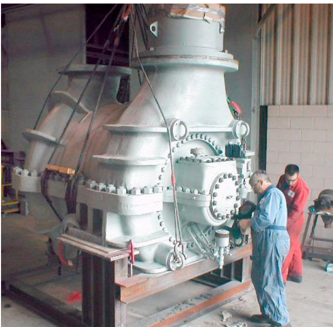
Complete refurbishment and reapplication of a Carrier compressor
