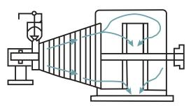
DOUBLE-FLOW CONDENSING accommodates high capacity steam flow for higher speed applications. The exhaust flow is split between two (2) duplicate rows of blades.
