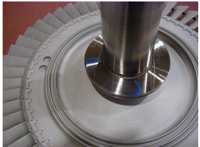
Repaired & rebladed rotor ready for installation
