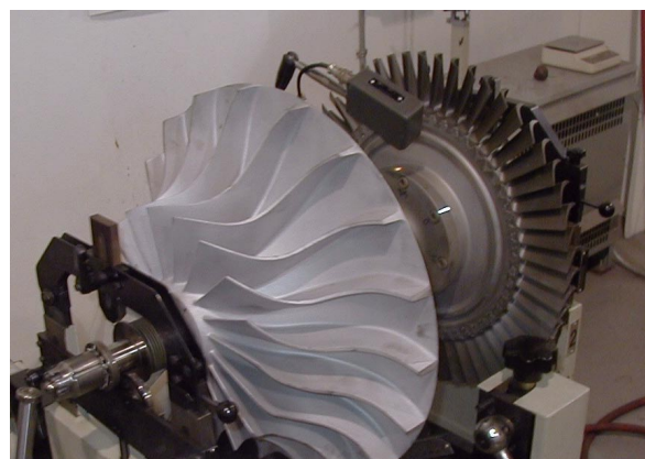
Repaired rotor ready for balancing
