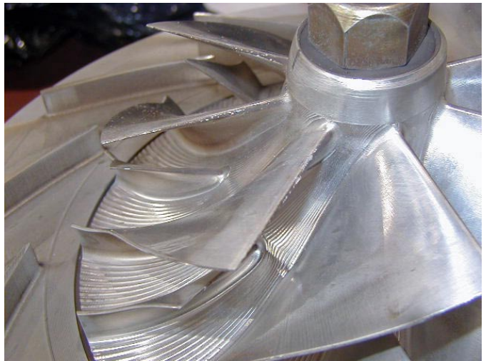
Air end impeller installed & ready for final assembly
