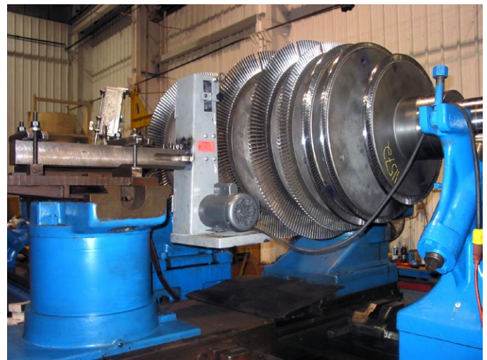
Tip grinding of blades
