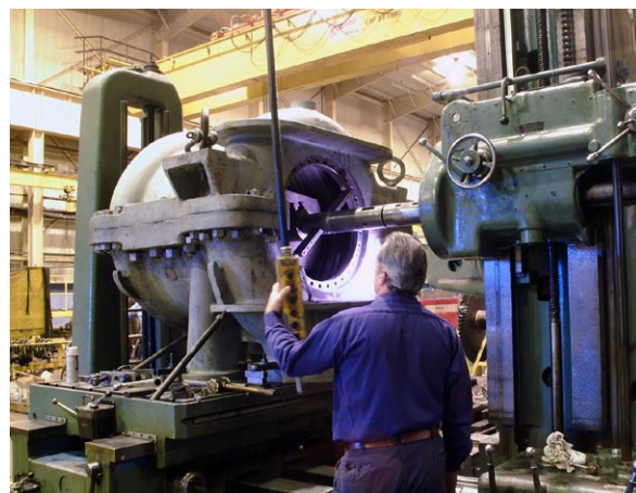
Complete compressor case and component restoration
