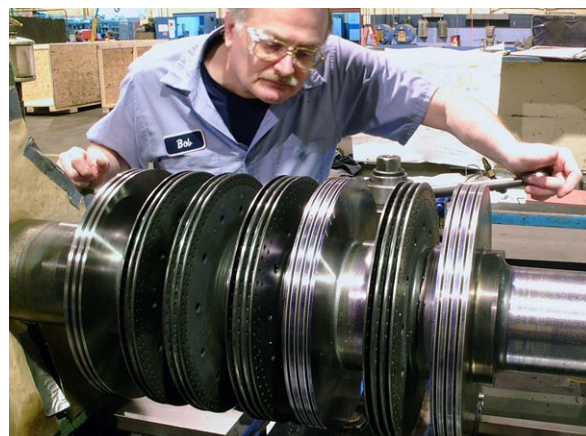
Weld repairing and re-machining of turbine disks and interstage labyrinth seals
