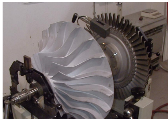
Repaired rotor ready for balancing
