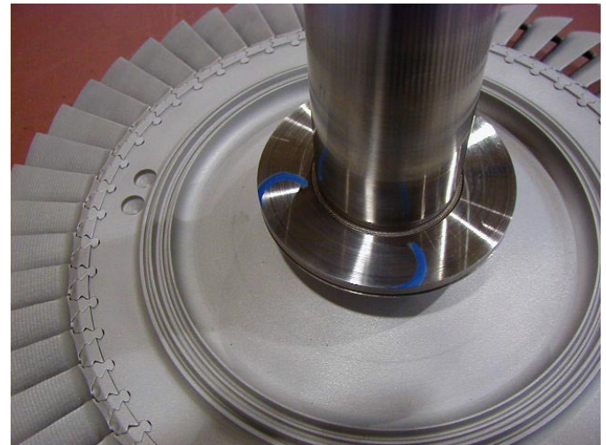
Repaired & rebladed rotor ready for installation
