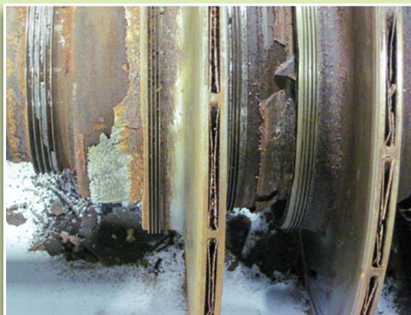
Figure 2. Fouling damage caused by salt carryover.
