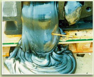
Figure 1. Foulant with tar-like consistency oozing from compressor.
