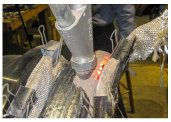
We can restore a rotor in a fraction of the time and a fraction of the cost of a new rotor, while maintaining mechanical integrity. Our weld restoration program combines the skills of our dedicated engineers, welders, and machinists; the results of comprehensive testing and analysis; and the reliability of our proven rotor restoration procedures to ensure the highest quality repair.
