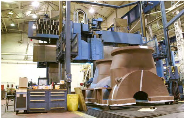
103M3 compressor casing on the masterhead.
