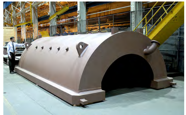
110M6 compressor casing.
