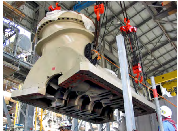
88M4 low-pressure mixed refrigerant pressure compressor casing.
