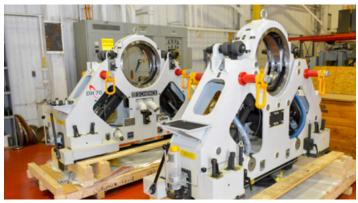
Bearing pedestals for rotors 27,500 to 44,000 pounds (12,474 to 19,958 kg).
