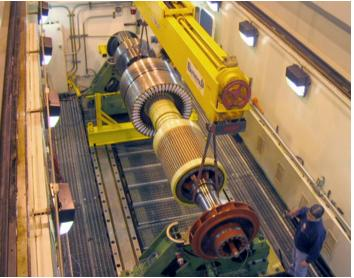
Exciter rotor weighing 19,000 pounds (8,618 kg) being lowered into bearing pedestals in preparation for high-speed balance.
