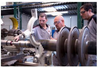
Inspecting a weld repair before balancing an Elliott steam turbine rotor.
