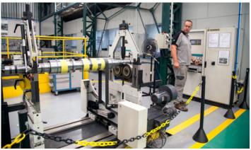
Balancing a new Elliott centrifugal compressor rotor shaft.
