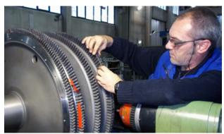
Reblading a turbine rotor.
