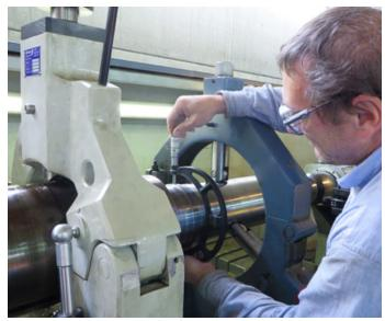
Measuring a compressor shaft at final machining.
