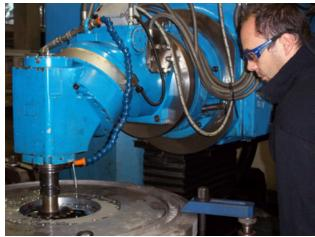
Machining a steam turbine diaphragm.
