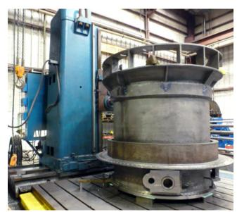
Elliott TH-140 hot gas expander inlet casing on large horizontal boring mill.
