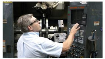
Turbine rotor forging in 30-inch CNC lathe.
