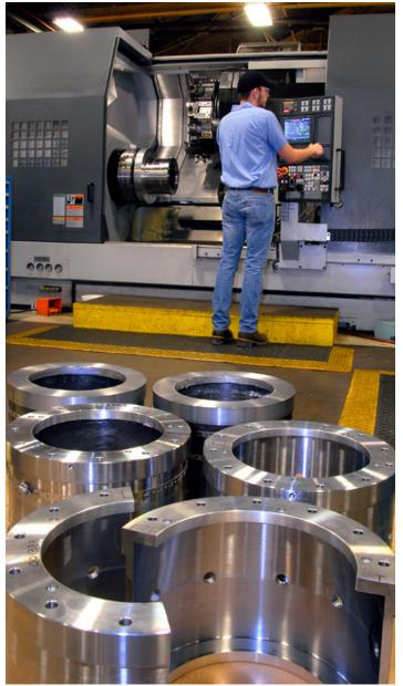
Machining various sizes of bearing components.
