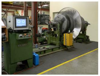
Balancing an Elliott SNV-16 turbine rotor on 40,000-pound balancing machine.
