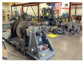
Machining an Elliott 103M compressor rotor on a 110-inch lathe.
