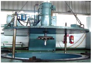
Preparing to balance an Elliott 25M impeller in a spin pit.
