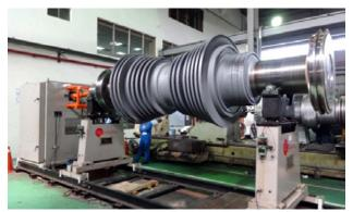
Balancing a 20.5-ton turbine rotor at Elliott Taiwan.
