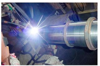
An Elliott technician TIG welding a turbine rotor.
