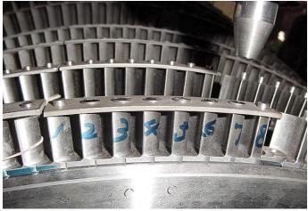
Peening a steam turbine rotor at Elliott Taiwan.
