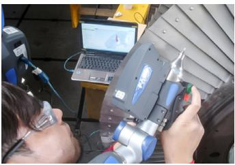
An Elliott technician measuring turbine blades using a FARO arm.
