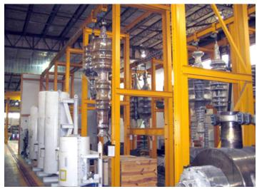
Rotor storage hanging capacity 10-ton x 18-feet long.
