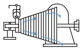
SINGLE-FLOW CONDENSING are highly economical and require the least steam for a given horsepower. Typically they are direct connected to a high-speed compressor.
