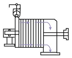
NON CONDENSING or BACK PRESSURE allow further use of the energy in the exhaust steam for process heat or other services.
