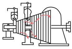
AUTOMATIC EXTRACTION and/or induction allows for controlled power and process steam pressure by automatically regulating the extraction/induction steam flows.
