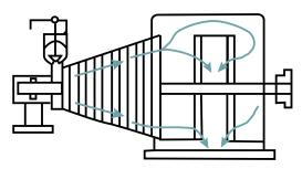
DOUBLE-FLOW CONDENSING accommodates high capacity steam flow for higher speed applications. The exhaust flow is split between two duplicate rows of blades.
