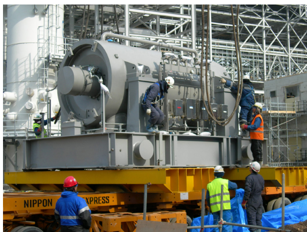
Figure 2. Elliott 60MB61 high pressure mixed refrigerant (HPRM) barrel compressor.
