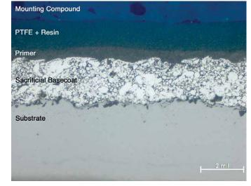
FIGURE 2 Cross-sectional photomicrograph of Pos-E-Coat system.
