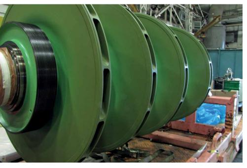
FIGURE Pos-E-Coat Plus coated rotor.
