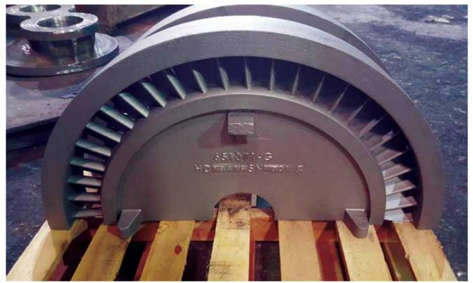
Each casting is half of a complete rotation. The first vanes on each half must be machined to marry up when assembled, so good dimenstional stability is needed.
