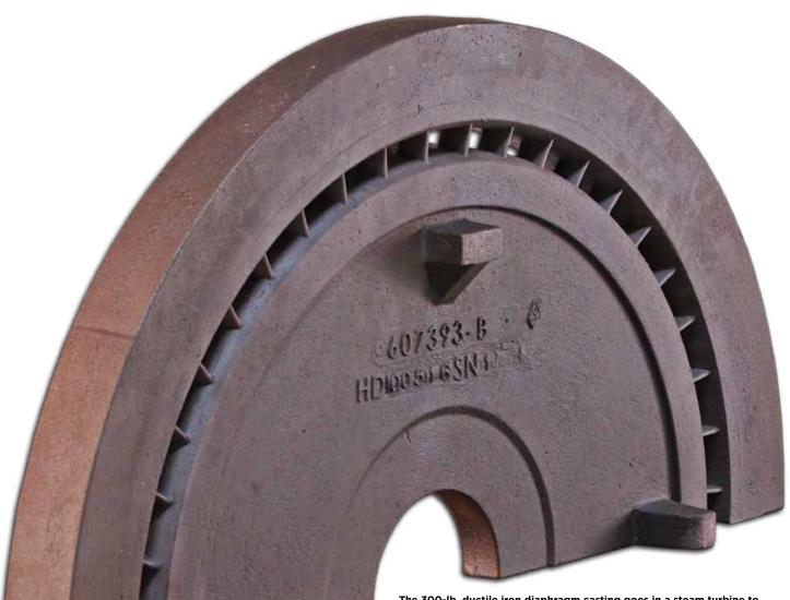
The 300-lb. ductile iron diaphragm casting goes in a steam turbine to help guide the inflow of steam.
