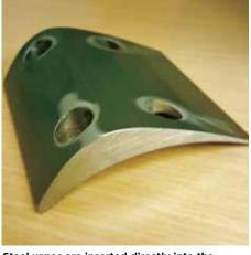
Steel vanes are inserted directly into the 3-D printed core and then the whole core package is placed in the drag part of the mold for pouring.
