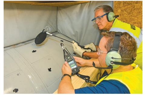
Figure 2. Noise measurement team collecting the sound intensity data inside sealed enclosure on the compressor casing
