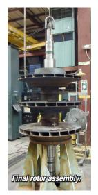
An overspeed spin test was required before final rotor assembly to verify the integrity of the repaired impeller. To minimize the turnaround time, Elliott transported the impeller by private airplane to the test facility 800 miles away. After successful testing, the impeller was returned to Jacksonville for rotor assembly, balance, and shipment to the customer for installation. Once the high-vacuum blower was back in service, the repaired rotor operated for a year without incident.
