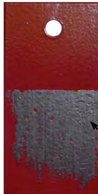
**FIGURE 7** Steel sample coated with proprietary imitation foulant used to test coating foulant release ability.
