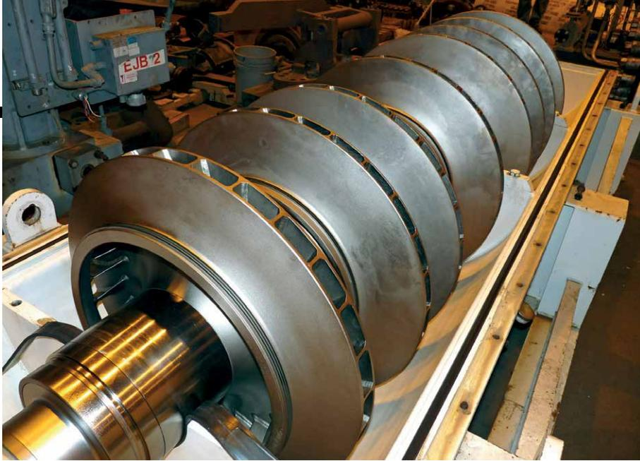
**FIGURE 5** Rotor coated with Pos-E-Coat 523 after six years of operation with the coating still intact.
