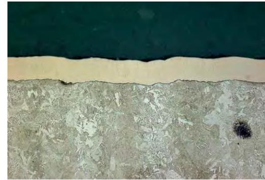
**FIGURE 6** Cross-sectional photomicrograph of Pos-E-Coat 523 system
