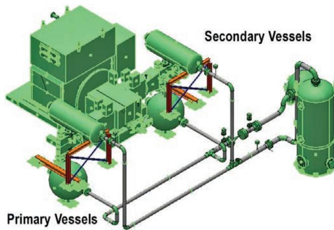
Figure 3. Example Pulsation Bottle Design For Hydrogen
