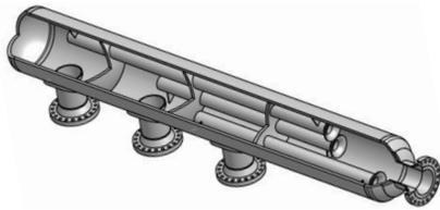
Figure 2. Typical Pulsation Bottle Design For Natural Gas
