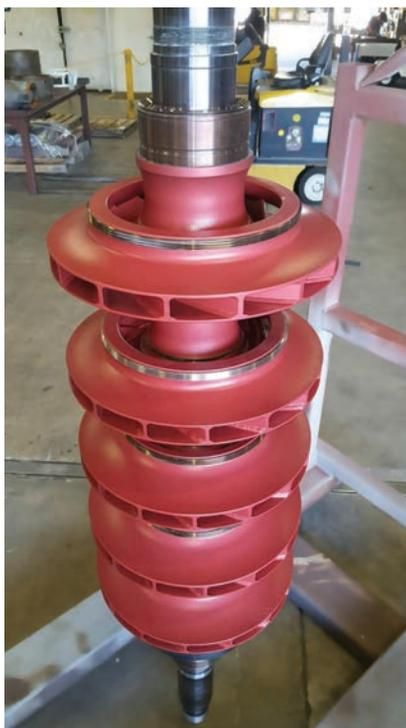
Figure 1. Specialty Pos-e-Coat Hydrogen Compressor Coating Developed By Elliott
