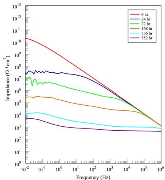
**Figure 4.** EIS test results in saturated ammonium chloride electrolyte for Coating 18 (left) and a coating that was permeated (right).
