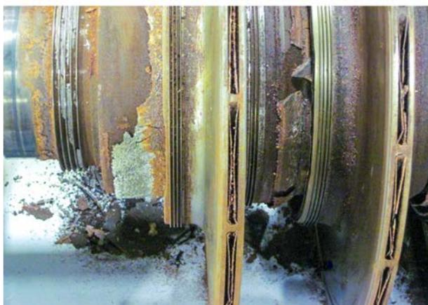
**Figure 1.** Examples of fouling caused by internal polymerisation (top) and salt carryover (bottom).
