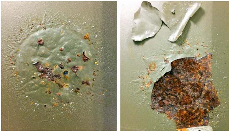
**Figure 5.** Exposed area of a permeated coating immediately after test (left) and after peeling back the coating to reveal the substrate (right).
