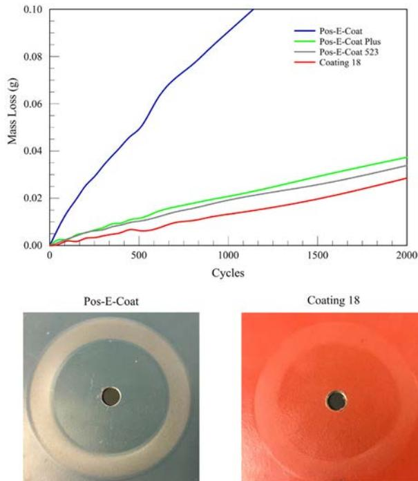
**Figure 3.** Results from wear testing using the Taber Abraser.
