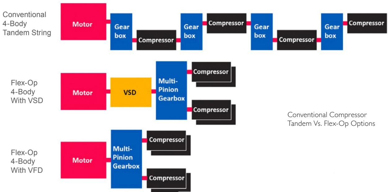
gear, which means the rotor speeds can be individually optimized for highest aerodynamic efficiency. Elliott's barrel casing configuration, coupled with the multi-pinion gearbox, allows the entire assembly to be powered by a motor with a variable frequency drive (VFD) or a motor in conjunction with a variable speed drive (VSD) for speed control.
