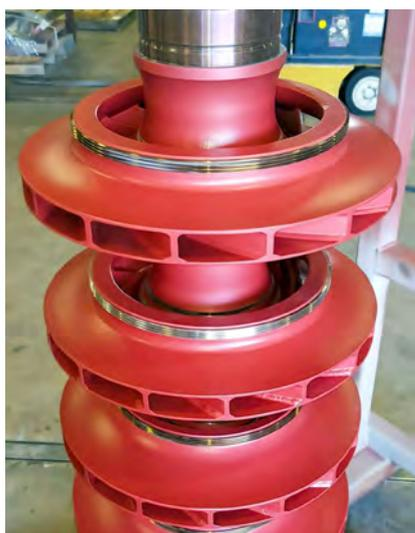
**Figure 2.** Specialty Pos-e-Coat® hydrogen compressor coating developed by Elliott.
