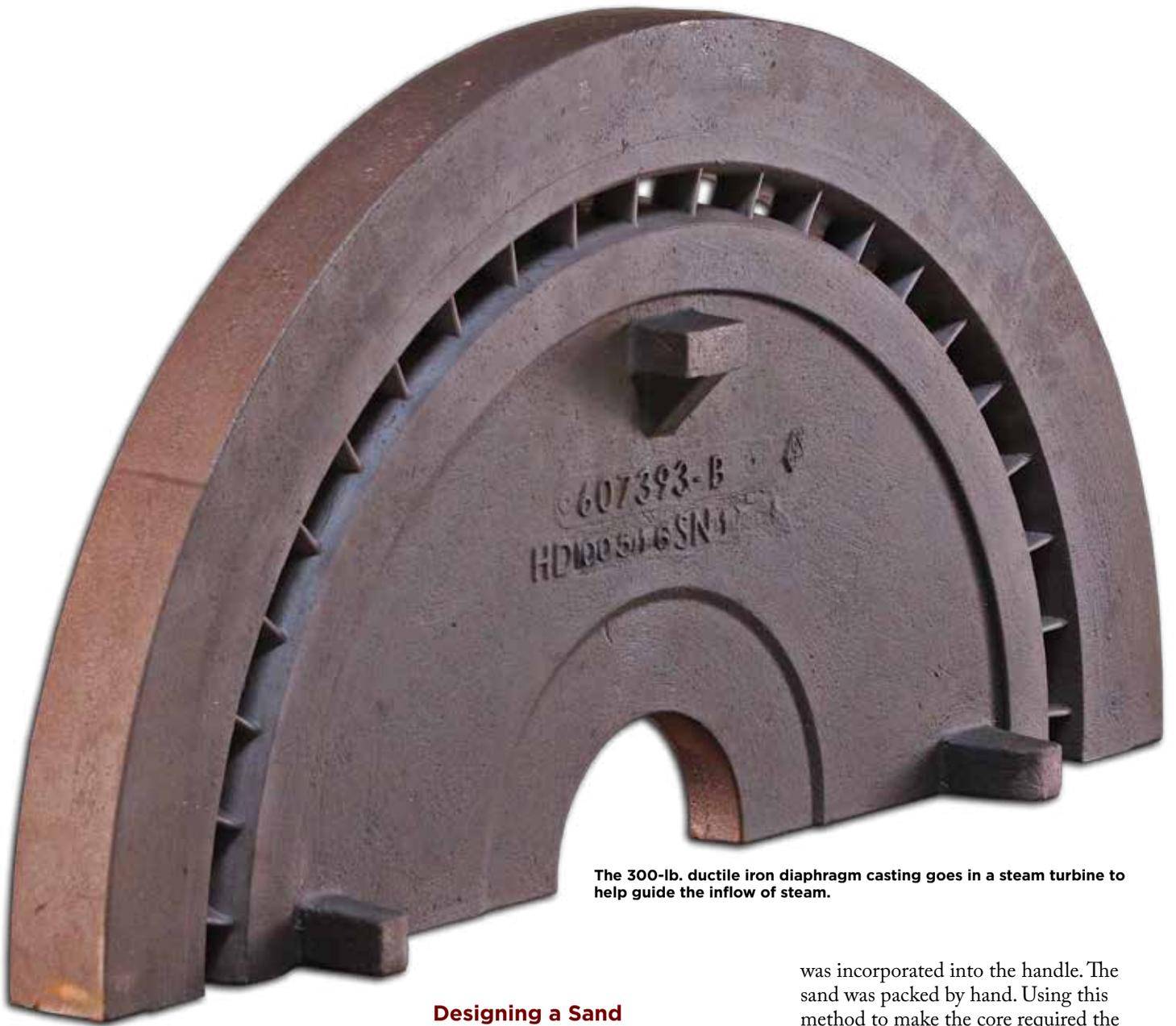
The 300-lb. ductile iron diaphragm casting goes in a steam turbine to help guide the inflow of steam.
