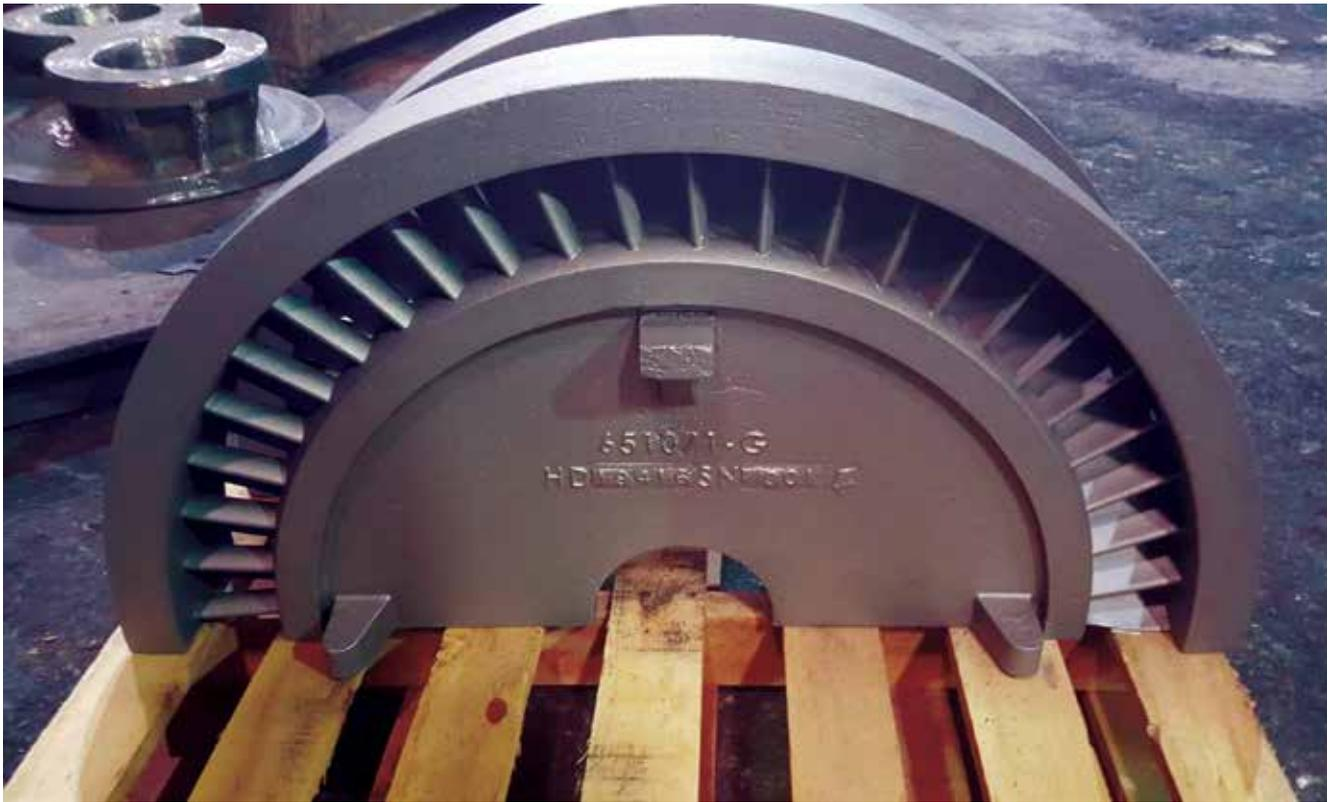
Each casting is half of a complete rotation. The first vanes on each half must be machined to marry up when assembled, so good dimensional stability is needed.
