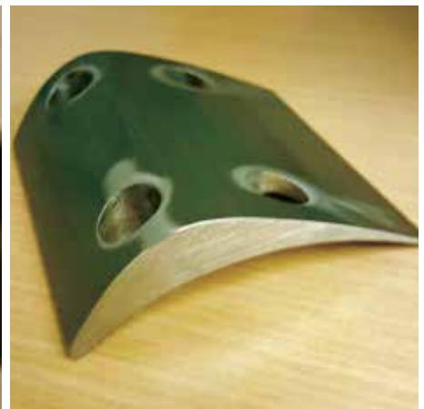
Steel vanes are inserted directly into the 3-D printed core and then the whole core package is placed in the drag part of the mold for pouring.
