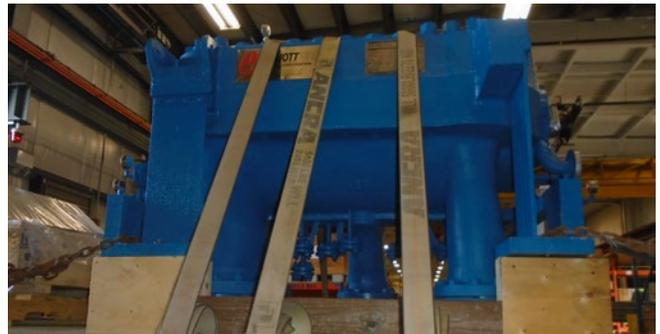
The overhauled ethylene refrigeration compressor loaded on a flatbed truck at the Burlington Service Center.
