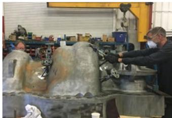
Elliott technicians modifying the HP compressor casing with new wash system injection points.
