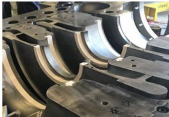
LP compressor upper casing with new interstage seals.
