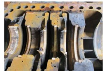
LP compressor upper casing prior to inspection and interstage seal replacement.
