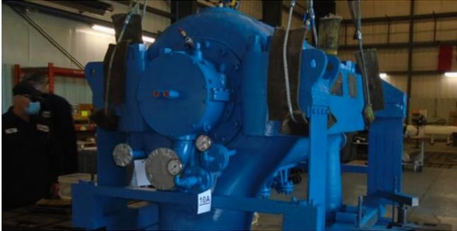
Ethylene refrigeration compressor after overhaul and coating application at the Burlington Service Center.
