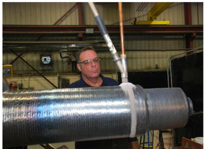
*Submerged arc welding of a 22-foot long, 39,000-pound rotor shaft.*
