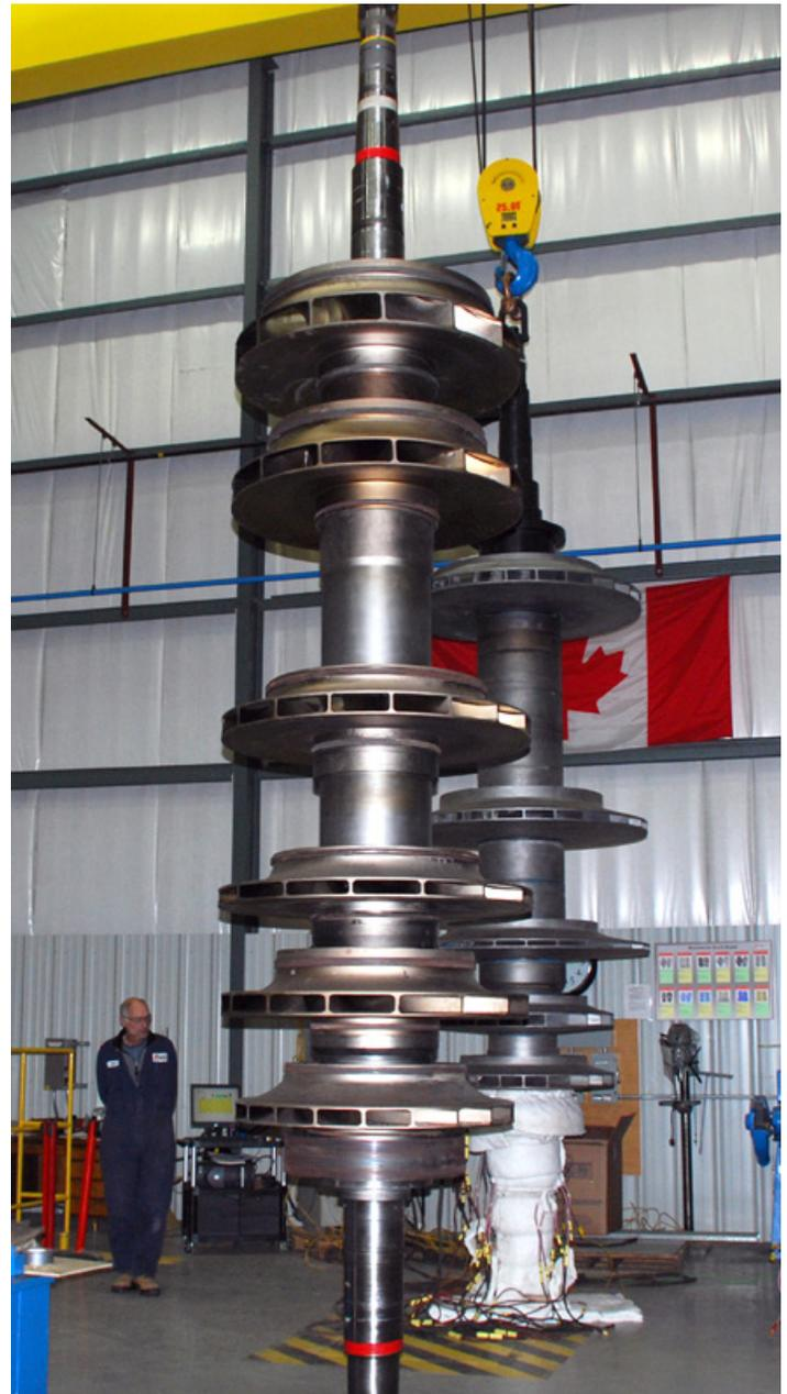
Front: Stacking an Elliott 70M compressor rotor.
