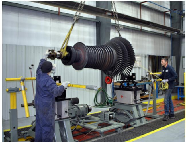
*Positioning a multi-stage turbine rotor onto 50,000 pound balance machine.*
