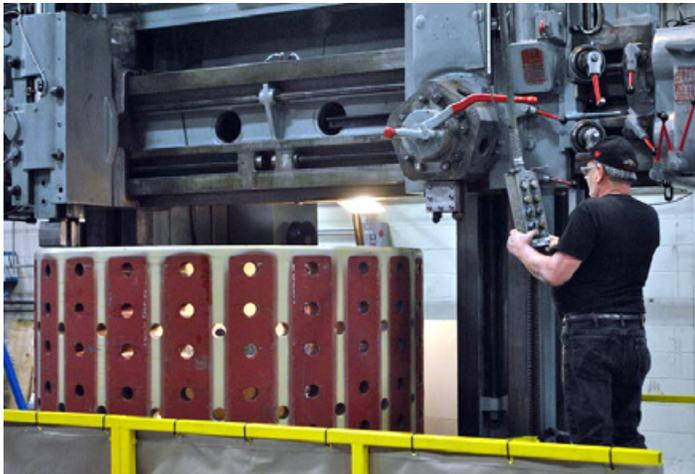
Machining a spider for an electric motor on a vertical boring mill.
