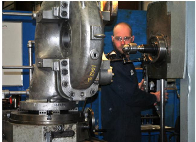
*Adjusting casing alignment on a horizontal boring mill.*
