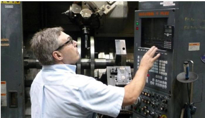
Turbine rotor forging in 30-inch CNC lathe.
