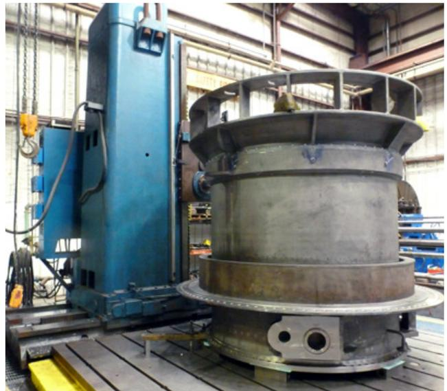
*Elliott TH-140 hot gas expander inlet casing on large horizontal boring mill.*
