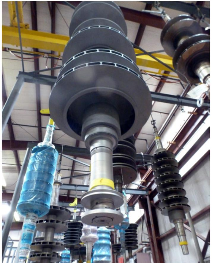
Climate-controlled, vertical rotor storage facility to protect and keep spare rotors readily available when needed.
