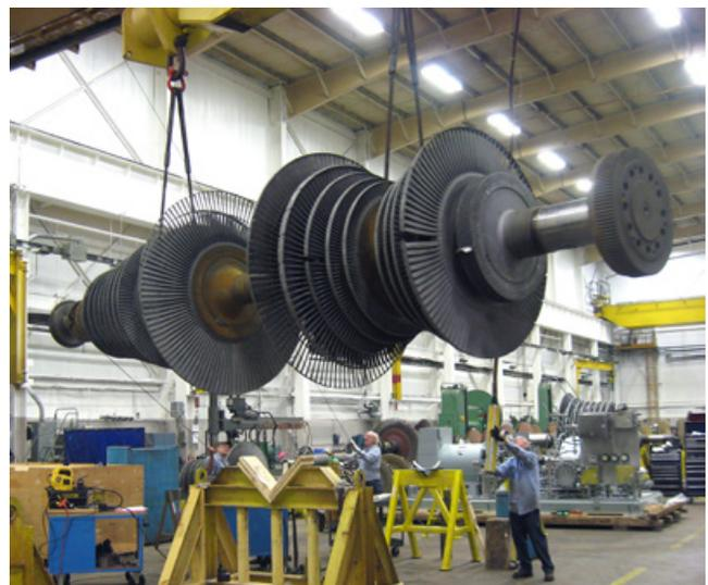
*Preparing a large, single- and double-flow, low-pressure rotor for a sling check.*
