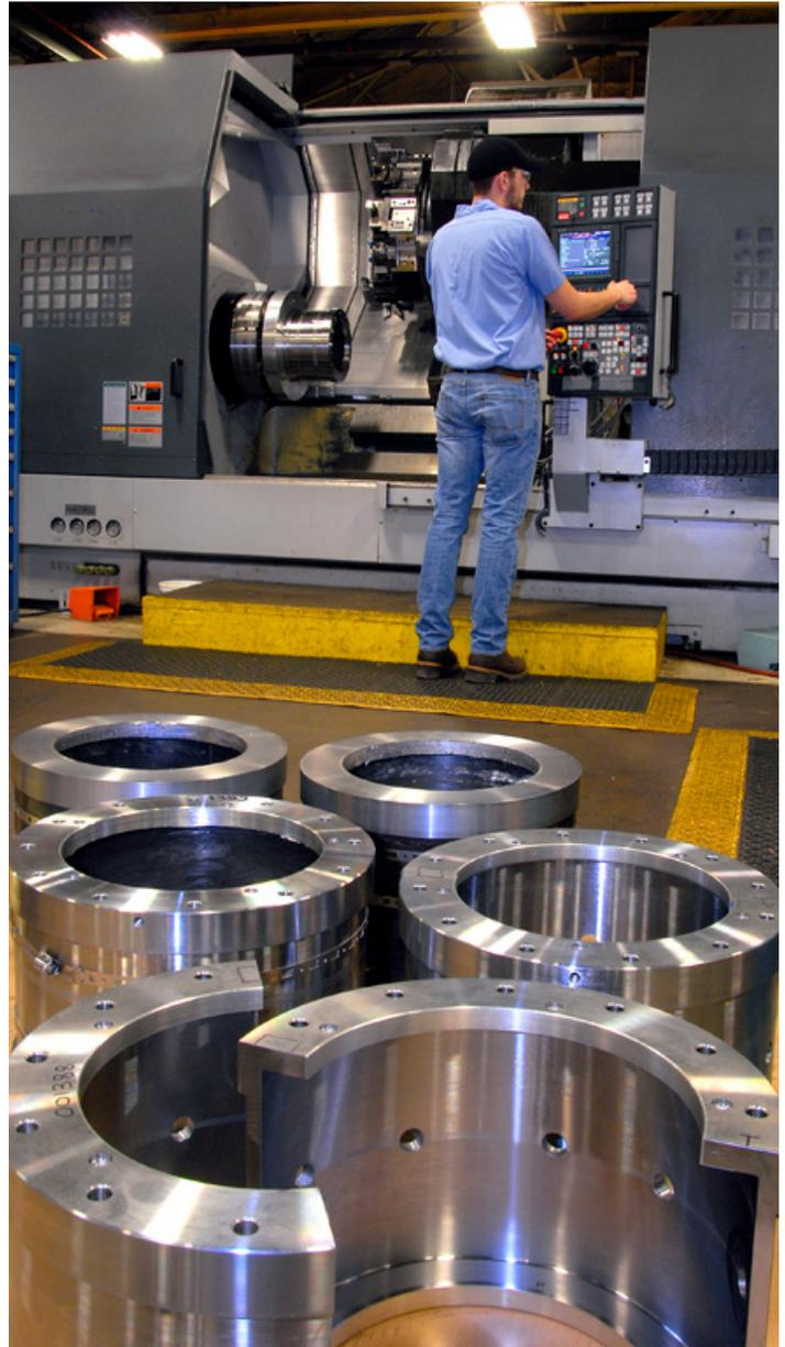
*Machining various sizes of bearing components.*
