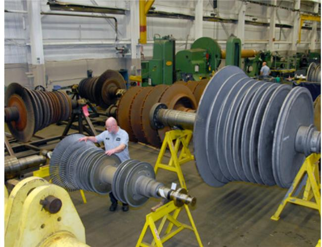
*Positioning a large multi-stage steam turbine rotor in inspection area.*
