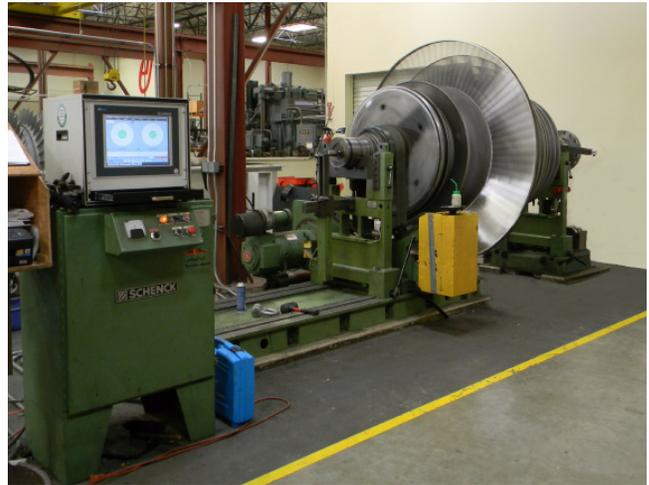
*Balancing an Elliott SNV-16 turbine rotor on 40,000-pound balancing machine.*
