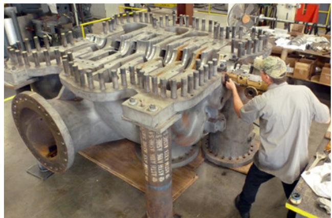
*Overhaul and reapplication of a non-Elliott compressor with Elliott components and nameplate.*
