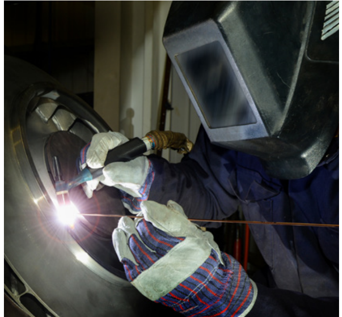
TIG weld repair of an impeller.
