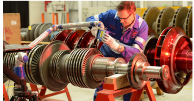
Using a portable coordinate measuring machine to reverse engineer a turbine rotor.
