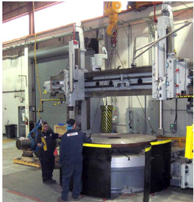
*Loading a disc to be machined to a thickness with a tolerance of (+/-) 0.001 inch.*
