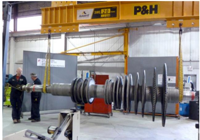
*Positioning a large multi-stage steam turbine rotor in inspection area.*
