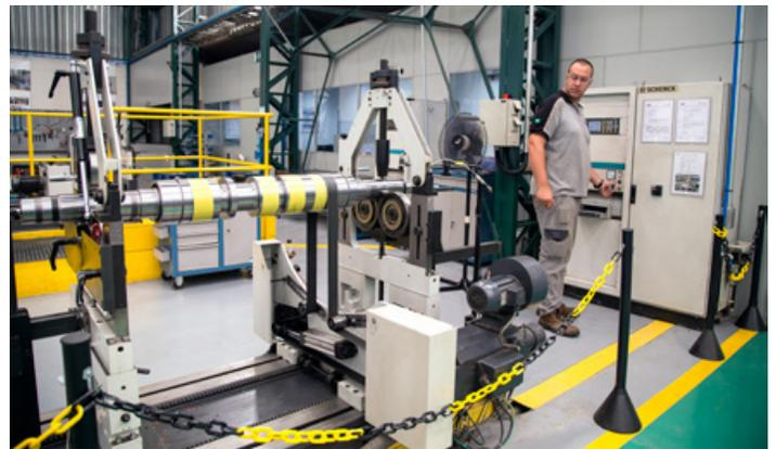
Balancing a new Elliott centrifugal compressor rotor shaft.
