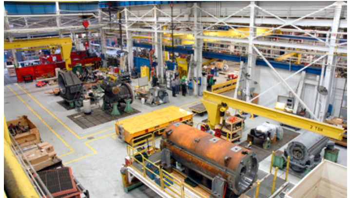
Assembly area for small and medium compressors and turbines
