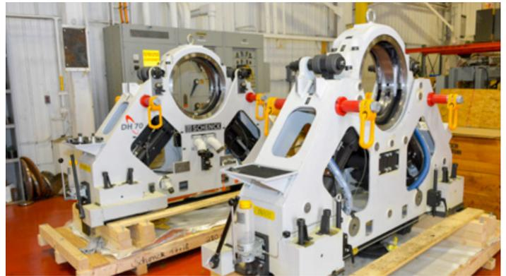
Bearing pedestals for rotors 27,500 to 44,000 pounds (12,474 to 19,958 kg).
