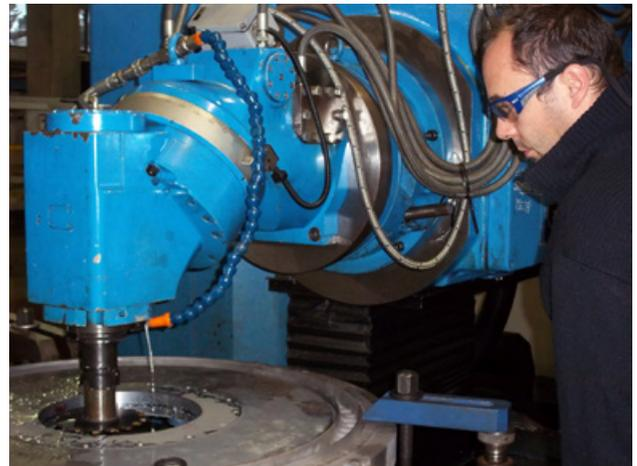
Machining a steam turbine diaphragm.
