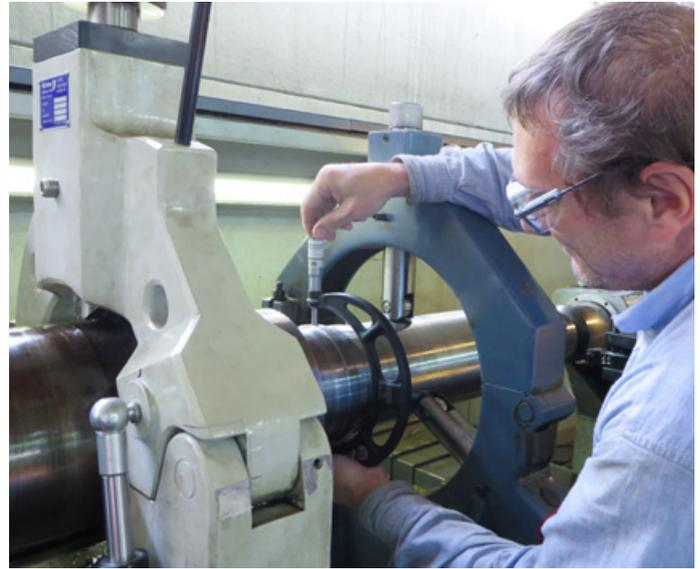
Measuring a compressor shaft at final machining.
