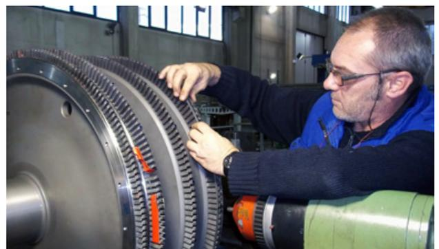
Reblading a turbine rotor.
