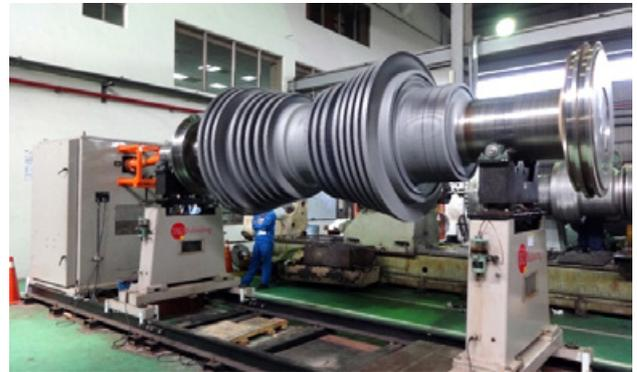
*Balancing a 20.5-ton turbine rotor at Elliott Taiwan.*
