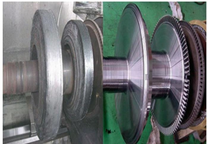
Disc buildup of a steam turbine rotor using submerged arc welding.
