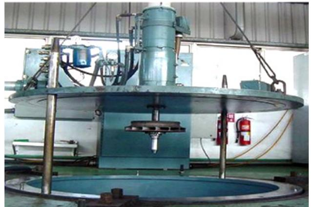
*Preparing to balance an Elliott 25M impeller in a spin pit.*
