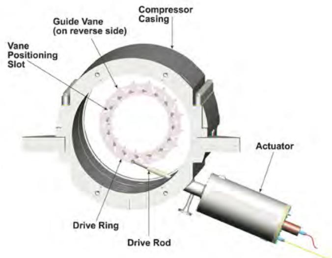
Elliott AIGVs are available for Elliott M-line centrifugal compressors, frame sizes 20M to 56M (~2,900 to 59,000 acfm).
