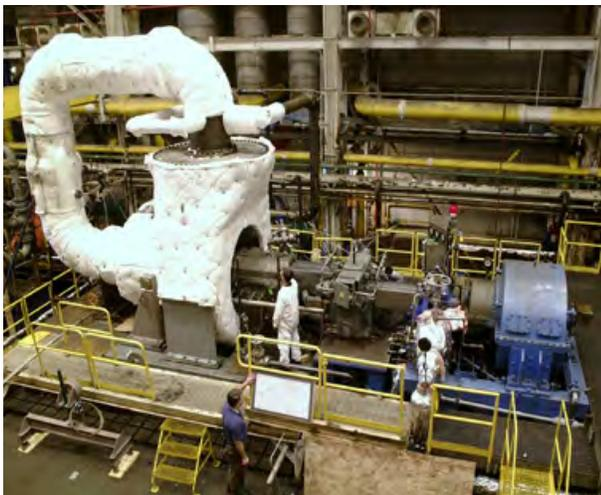
Hot mechanical test of TH expander.
