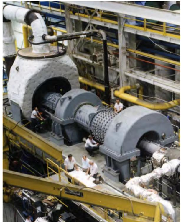
*Testing an axial compressor.*
