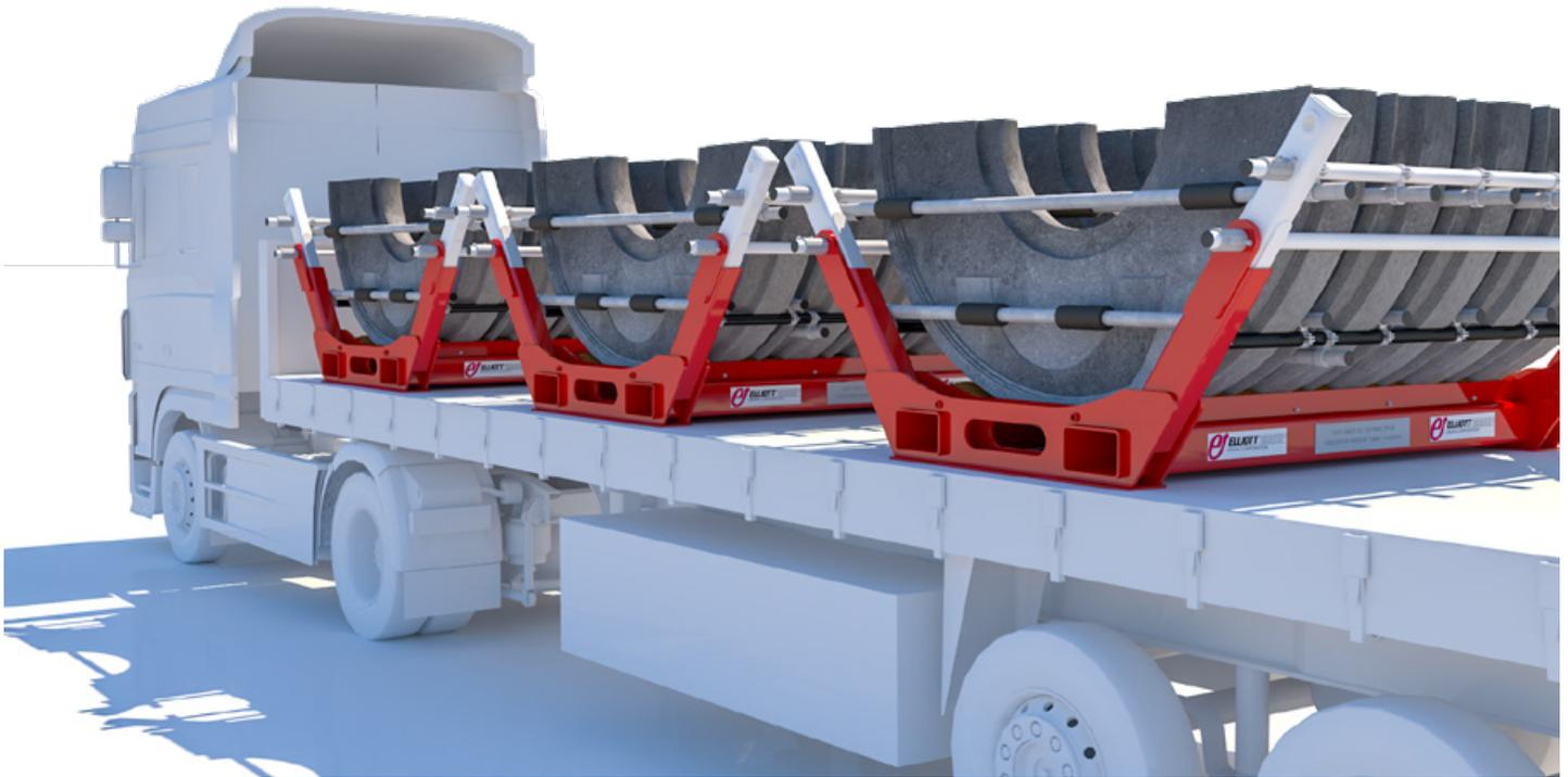
Full diaphragm storage rack containers loaded onto a truck for transport.
