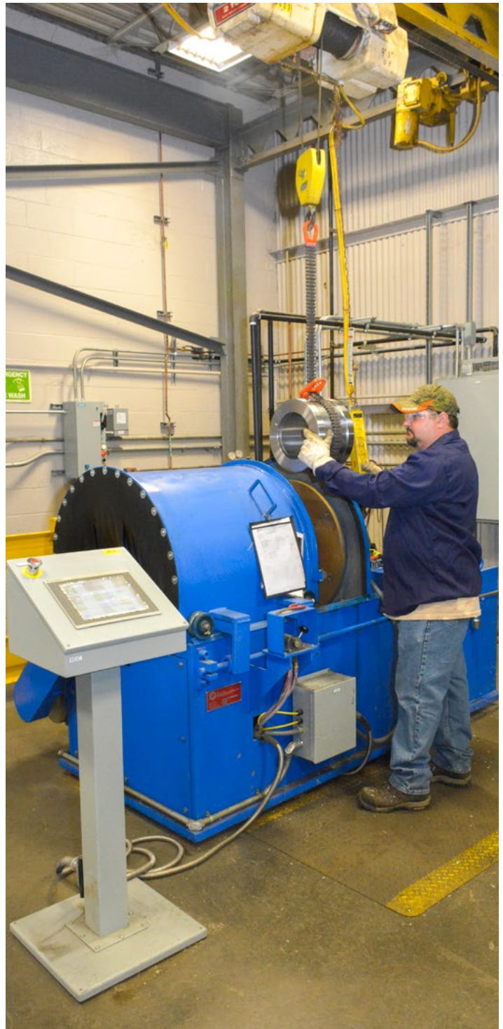
Centrifugal babbitt casting.
