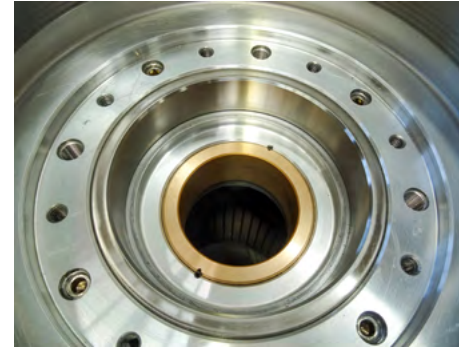
Replacement of casing wear ring.
